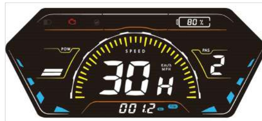
Figure 1-Fault warning display interface
